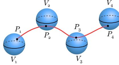
Figure 2: Relaxed path  $RelPath_{EF} = (V_1, \dots, V_4)$  that consists of spheres and path  $Path_{EF} = (P_1, \dots, P_4)$  that belongs to it. Smooth function of the end-effector movement is depicted with red curve.
