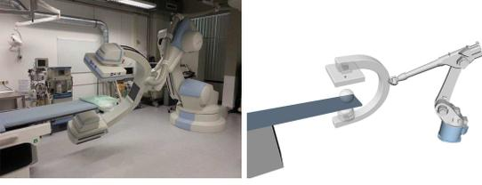
Figure 3: Layout of the robot equipped with C-arm.
