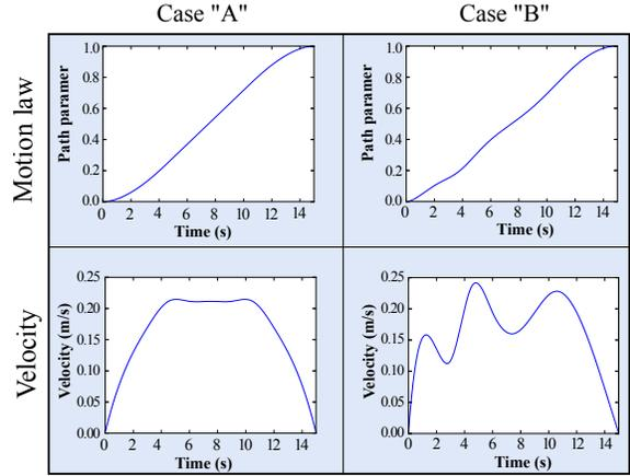
Figure 5: Given motion laws and computed end-effector velocities.
