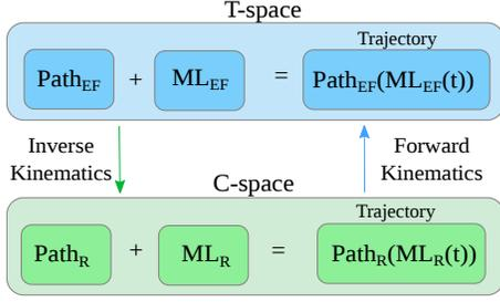
Figure 1: Overview of the robot trajectory calculation.
