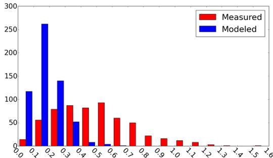
Fig. 4. Distance error (mm) frequency plot of *RotXYZ-TransXYZ-error positional model*
