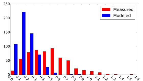
Fig. 2. Distance error (mm) frequency plot of *RotZ-error* positional model
