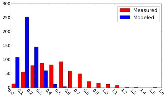
Fig. 3. Distance error (mm) frequency plot of *RotXYZ-error positional model*
