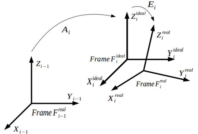
Fig. 1. Frame transformations in presence of errors
